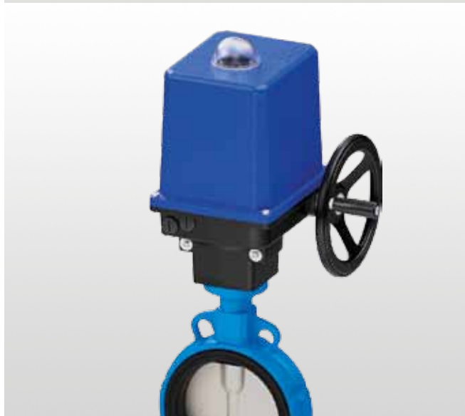
S301 ISO5211 with 230V-50Hz one phase or 400V-50Hz three phases IP67 electric actuator
