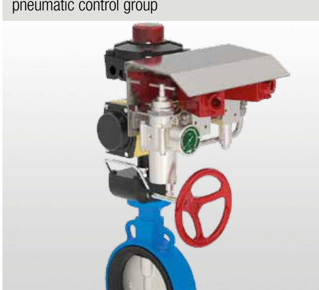
S301 ISO5211 with disengageable gear box, pneumatic actuators, limit switch box and pneumatic control group
