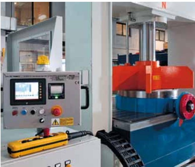
Vertical hydraulic test machine. For butterfly and ball valves.
