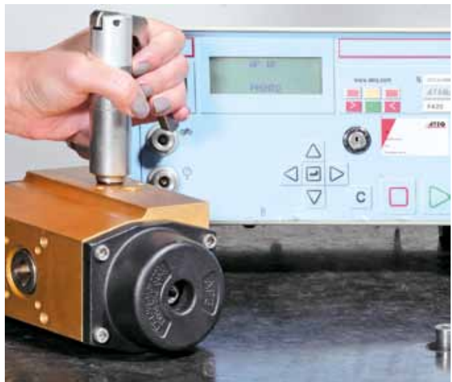
Leak test machine. For pneumatic rotary actuators.
