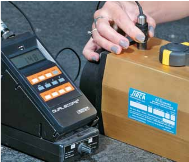
Coating thickness gauges. For coating thickness measurement on metals.
